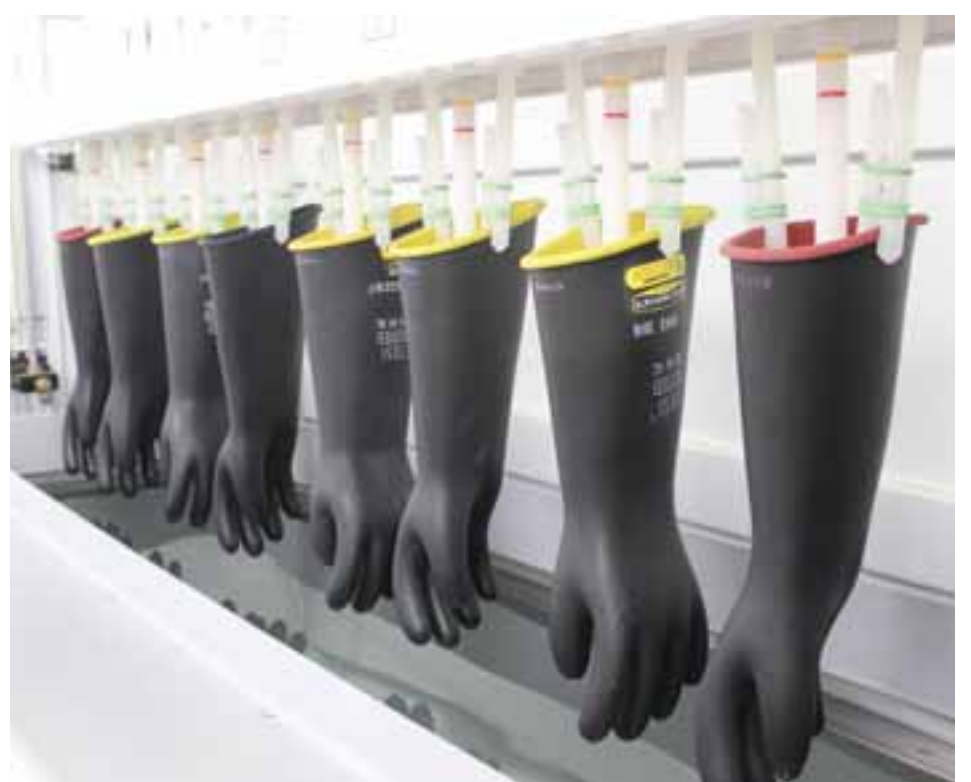
The staff cleans and scrutinizes each item for visual signs of wear and tear before subjecting them to electrical testing.
