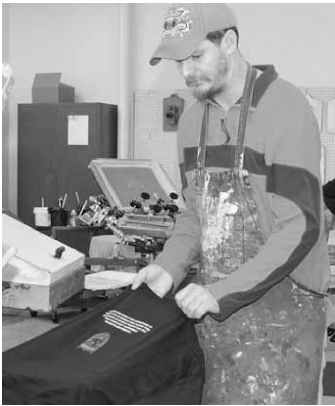
T.J. Vandagriff, an employee at Power Print, pulls a freshly screen-printed shirt from the press to transfer it to a dryer.
