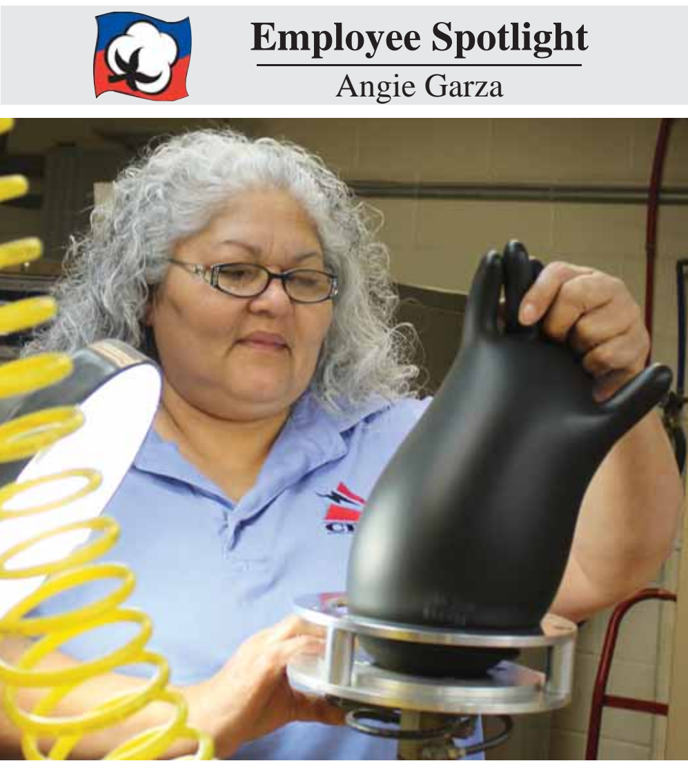
Angie Garza inspects a glove in the test lab of Cotton Electric Services, Inc. She reckons she has inspected about three-quarters of a million gloves for damage. Regular inspection of gloves and other protective equipment is an important safety measure for electrical workers. Inflating the glove magnifies any flaws. She laughed and said occasionally a glove will pop off the base of the inflator and once flew across the work table to slap a co-worker.
