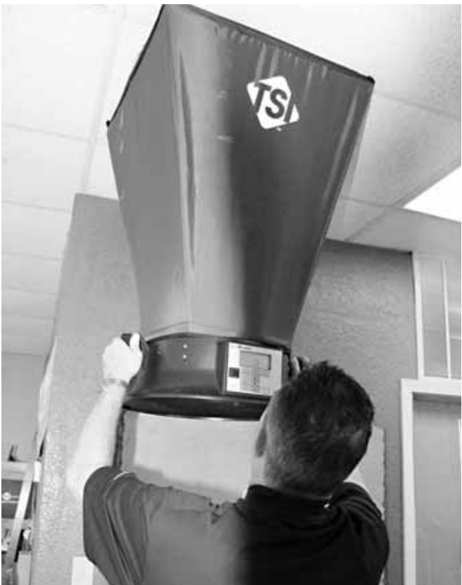
Bill Gorley uses an air flow capture hood to adjust settings for maximum comfort.
