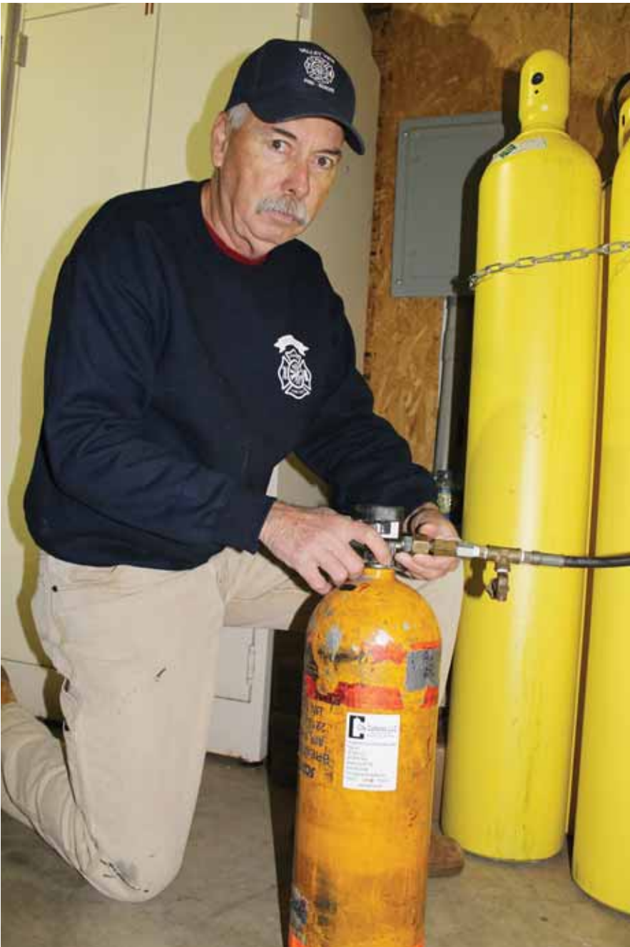
Fire Chief Lin Newton shows how members of Valley View Volunteer Fire Department will refill spent air canisters at fire scenes using a cascade system. The system and trailer to carry it were funded with a Cotton Electric Charitable Foundation grant.
