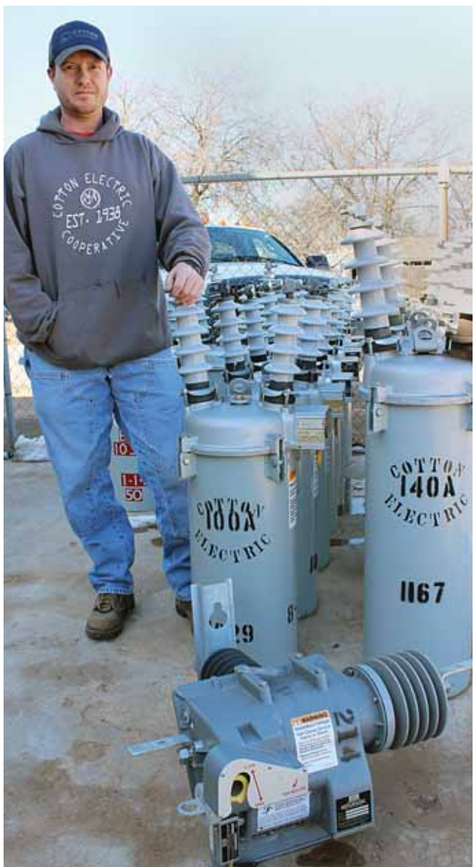
Devices on poles are larger than they appear. The top and middle photos show suspended electronic and oil-circuit reclosers, respectively. Below, apparatus technician Zac Hoodenpyle stands next to the same equipment. Zac works with reclosers, transformers and more, as explained in the Employee Spotlight on Page 6.
