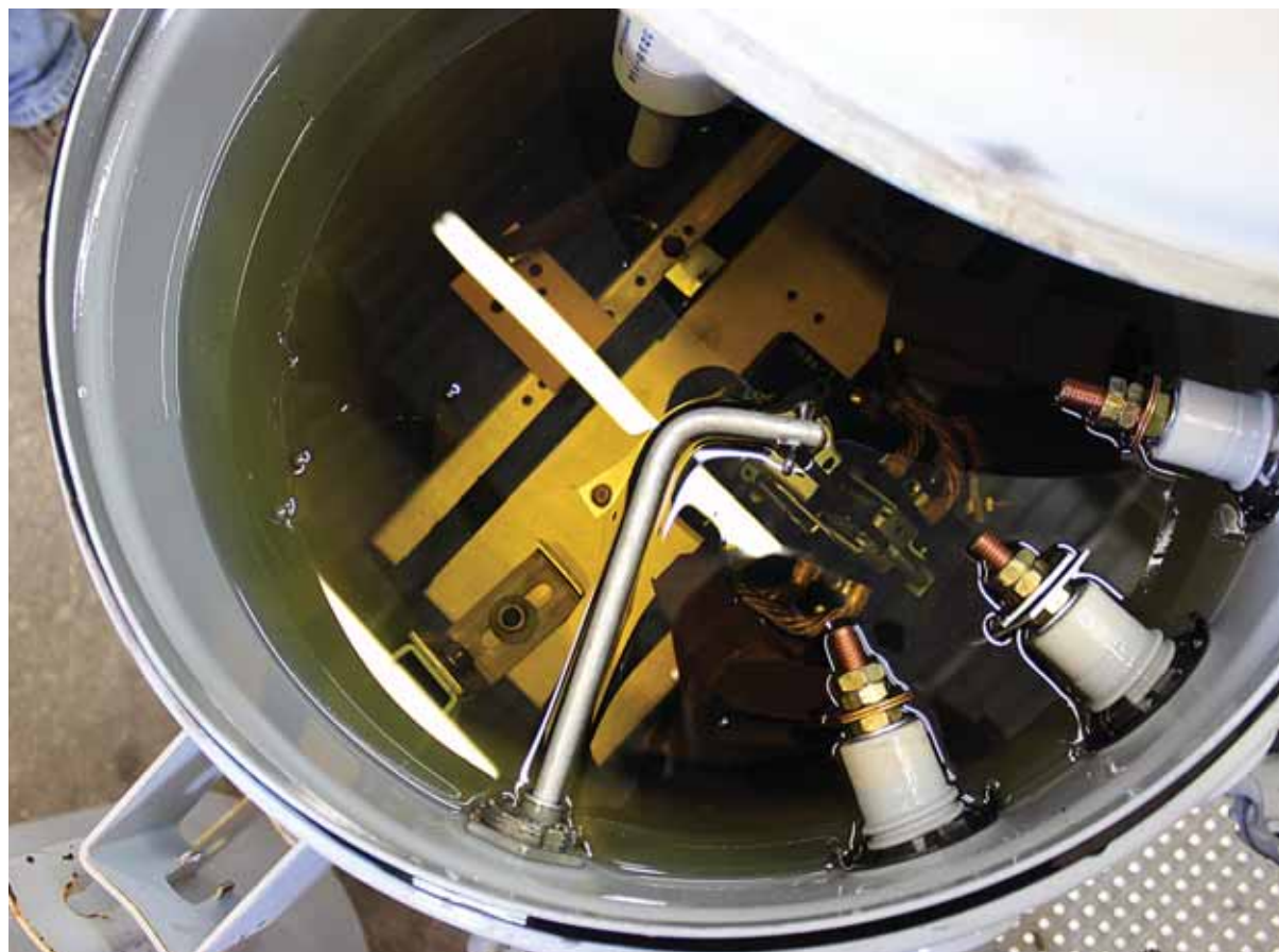
At left, Zac Hoodenpyle begins the refurbishing process by opening up transformers. The parts inside, above, are immersed in a non-conductive oil.
