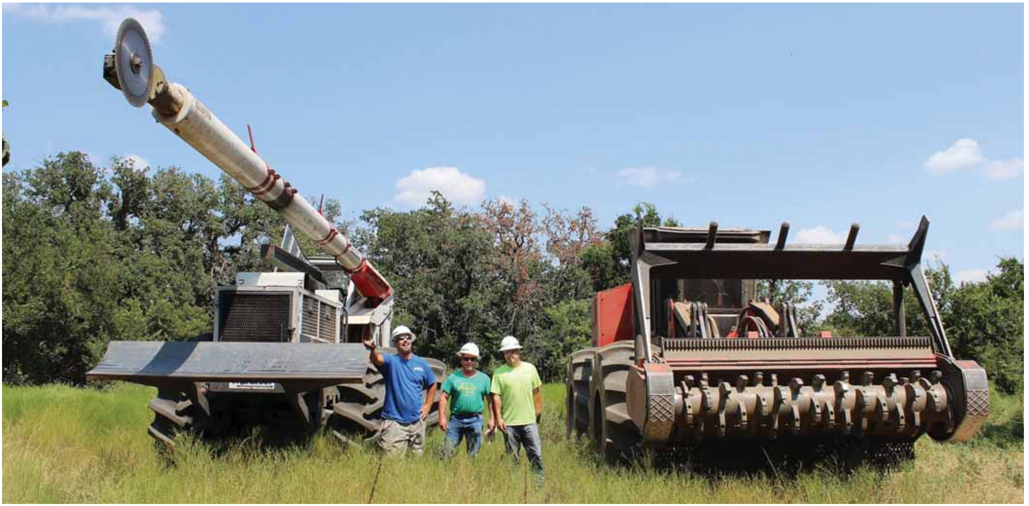
Workers on the NRS right-of-way clearing crew include, above from left, crew foreman Don "Gator" Butcher, TJ O'Conner and Justin Barnes. Machinery includes the Kershaw telescoping trimmer on the left and a rotary ax. In the photos below, the rotary ax begins and finishes work to take down a tree in the co-op's right-of-way.
