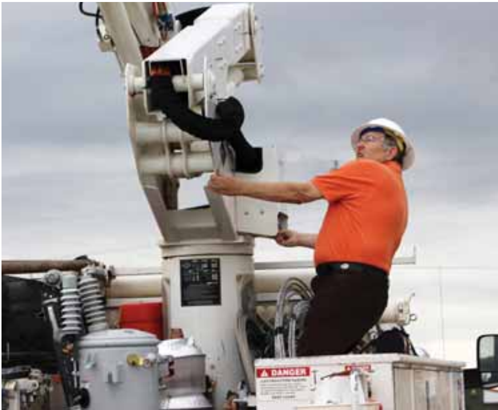
Larry Phillips, safety director for Cotton Electric, watches the basket as he performs the rescue drill.
